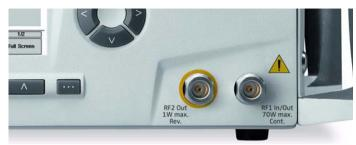
**RF2 OUT** is a 50  $\Omega$  N-type connector (female) on the front panel. It can be used to feed a signal into the receiver section of the unit under test (for example, a TETRA base station).
