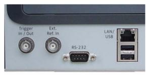
This 9-pin sub-D connector on the rear panel of the 2305 Stabilock can be used to control the 2305 remotely via a serial interface (RS-232). The command set and the responses conform to the SCPI standard and are explained in the user guide.
