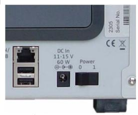
The 2305 Stabilock can be operated either from the internal battery or from an external DC source such as the power supply which is delivered with the 2305, or a car battery. The DC voltage must be in the range from 11 to 15 V. In addition, the battery is loaded when an external DC source is connected.
