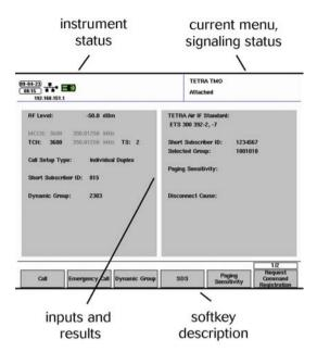
The top row shows the instrument status on the left. This includes the status of battery, network and USB connections.
